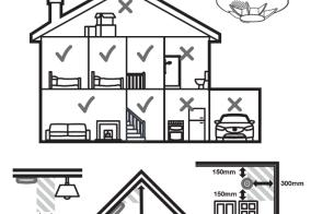
If positioning your smoke alarm on the wall, the top of the detection element must be between 150mm and 300mm below the ceiling, and at least 300mm from any neighbouring wall.
